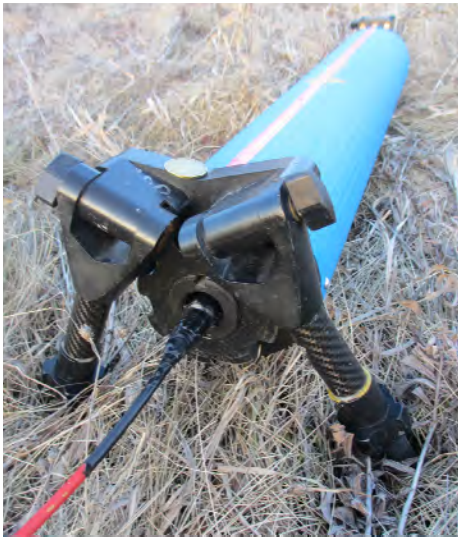
Figure 9: UTEM 5 sensor with field tripod legs attached. The fibre optic cable (red) is 9 m long and connects to the UTEM 5 receiver.
