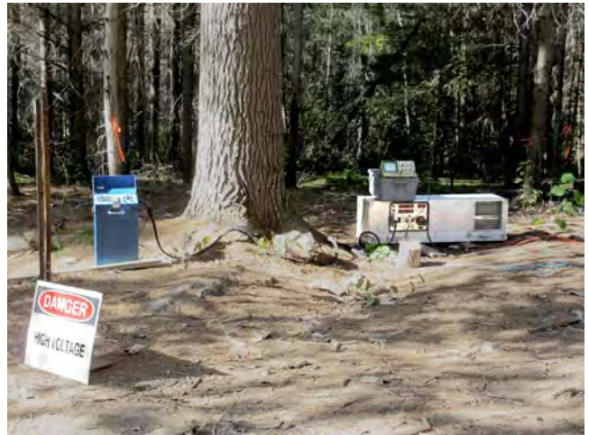
Figure 5: UTEM 4 transmitter setup. The control unit on the left is connected to the 1.4m long power mainframe unit by a cable of multiple optical fibres. The 11kW power generator is off the photograph.
