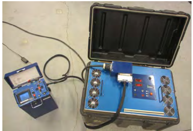
Figure 6: The UTEM 5 transmitter prototype. The control unit on the left is >3 m away from the power mainframe during operation. A 30cm ruler shows the scale
